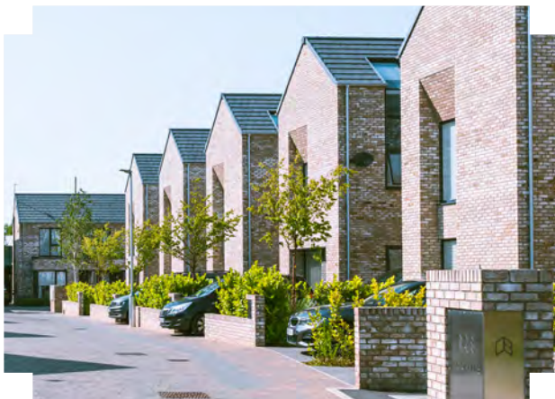
Subtle changes in surface material and a level surface contribute to a pedestrian-oriented residential street The Gables, Crosby
