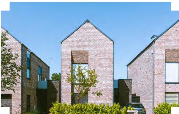
Staggered upper storey windows and narrow footprints prevents overlooking and allows a tighter block. Private terrace integrated to the side of each home. | The Gables, Crosby
