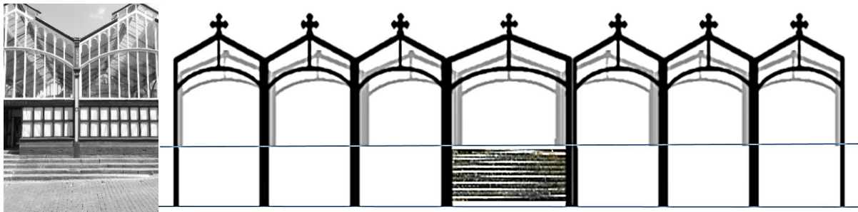
Stockport; Market Hall arcades. Cast iron. Elevation of proposed arcades for Adlington Square
